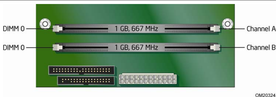
Figure 13. Dual Channel Memory Configuration Example
