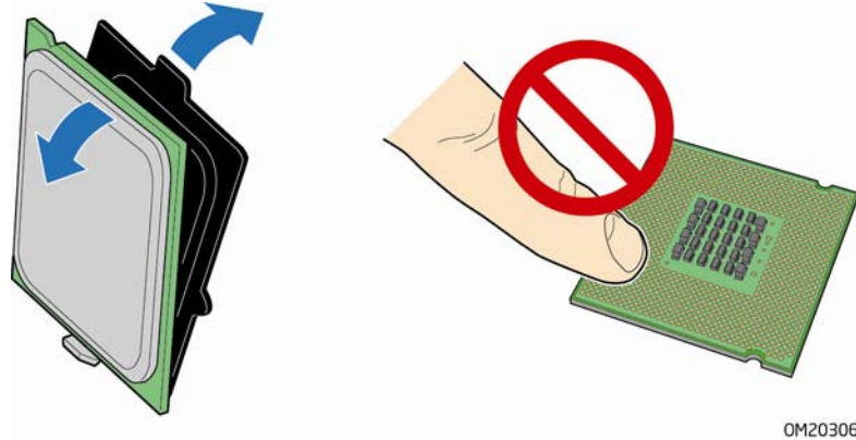
Figure 9. Remove the Processor from the Protective Processor Cover
