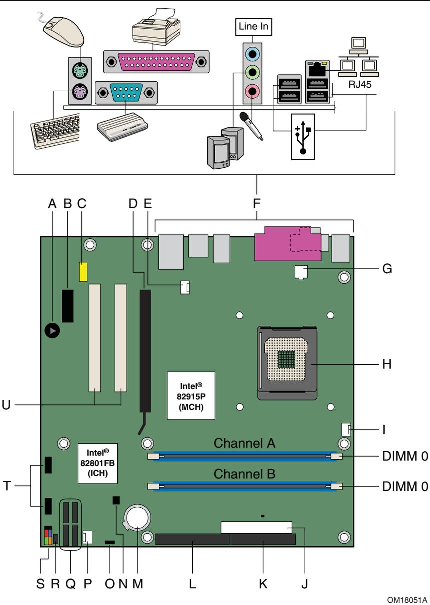
Figure 1. Intel Desktop Board D915PDT Components
