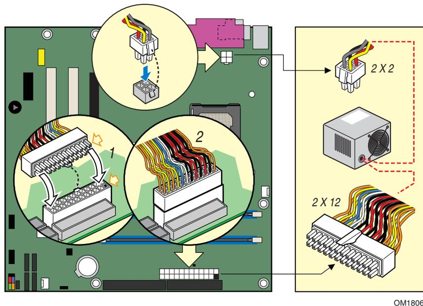
**Figure 21. Connecting Power Supply Cables**
