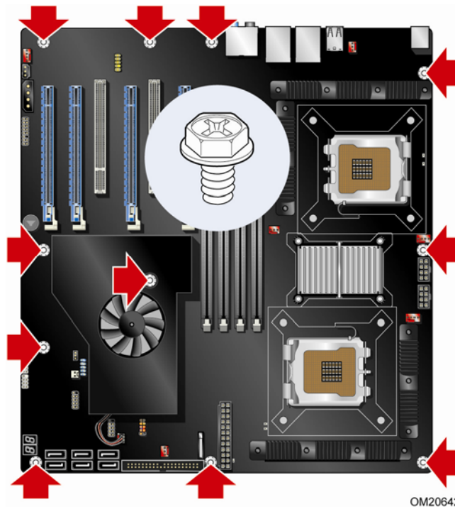
Figure 8. Desktop Board D5400XS Mounting Screw Hole Locations
