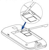
3. Slide the SIM card out from the slot with your other thumb or finger.
