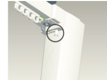
The latch hasn't pushed into the locked hole
