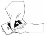
3. Insert the SIM card with the metallic part facing down and the clipped corner in the same direction and orientation shown on the cover's instruction.
