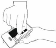
4. Insert the battery back to the battery slot.
