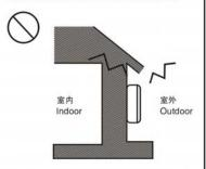
不正常燃燒可能導致生火或熱水爐被雨水破壞。 A fire may be caused by an abnormal combustion or the heater may be damaged by the rain.
