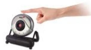
You can use the snapshot button to capture still images or rotate the lens cover to adjust the focus.
