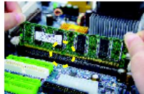
2. Insert the DIMM memory module vertically into the DIMM slot. Then push it down.
