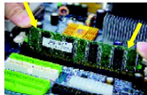
3. Close the plastic clip at both edges of the DIMM slots to lock the DIMM module. Reverse the installation steps when you wish to remove the DIMM module.
