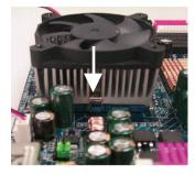
Fasten the heatsink supporting-base onto the CPU socket on the mainboard.
