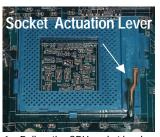
1. Pull up the CPU socket level and up to 90-degree angle.
