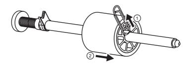
8. Attach the new pick roller to the shaft.
