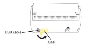
2. Connect the USB cable to the USB connector on the ScanSnap, and the other end of the USB cable into the USB port on your personal computer.
