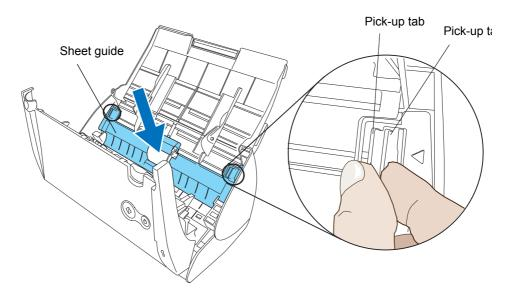
⇒ The sheet guide makes a clicking sound when the knobs fix into position.
