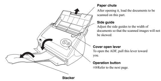
Before using the stacker, unfold and extend it as shown above.
