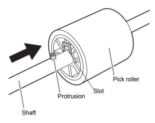
9. Install the pick roller with it's shaft to the scanner.
