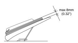
After the read command is issued from the host system and the documents are read, scanned documents are expelled into the stacker for removal.
