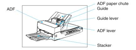
Fan the sheets before setting a stack of documents on the ADF paper chute.
