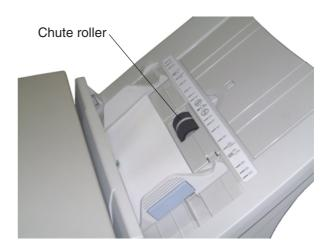
After the read command is issued from the host system and the documents are read, scanned documents are expelled into the stacker for removal.
