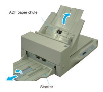
Set the guides so that there is a small clearance between the document edges and the guides. Load the document face down on the ADF paper chute and adjust the guides to the document width.
