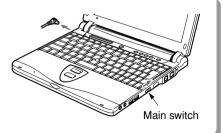
Slide the MAIN switch to the direction of the arrow ( ] side). ( ( ) lights up.
