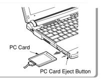
Press the PC Card Eject Button and remove a PC Card.
