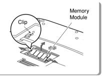
Pull clips sideways from each side of the memory and remove the memory module.
