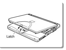
Press the front latch to unlock and open the LCD Display.
