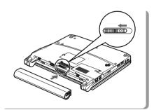
Align the groove on a battery pack with the projection on your PC and install a battery pack, then slide the Battery Pack Lock to lock it.
