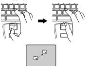
Dragging means, while keeping the upper button depressed, moving the mouse pointer by pressing the stick to the desired location and releasing the button.
