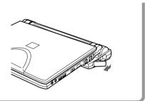
Pull the connector box removing lever toward the arrow direction to unlock.
