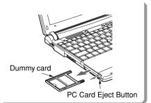
Press the PC Card Eject Button and then pull a dummy card out of the slot.
