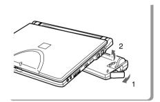
(1) Pull the removing lever and (2) lift your PC up and detach the connector box.
