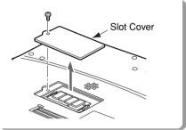
Remove the RAM Expansion Module Slot Cover on the bottom side of the PC.
