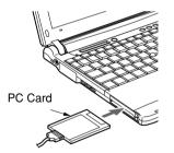
When the PC Card is installed for the first time, install a driver if necessary.
