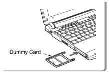
Insert a dummy card fully into the PC Card Slot.
