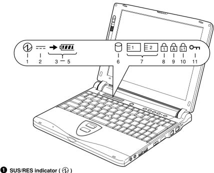
This indicator appears up when this PC unit is functioning and blinks when the unit is in suspend status.
