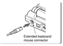
Connect a mouse to the extended keyboard/ mouse connector on the connector box. Connect it with the engraved arrow mark facing up.
