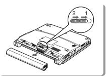
(1) Slide the Battery Pack Lock to unlock and (2) while sliding the Battery Pack Removing Button, remove the battery pack.
