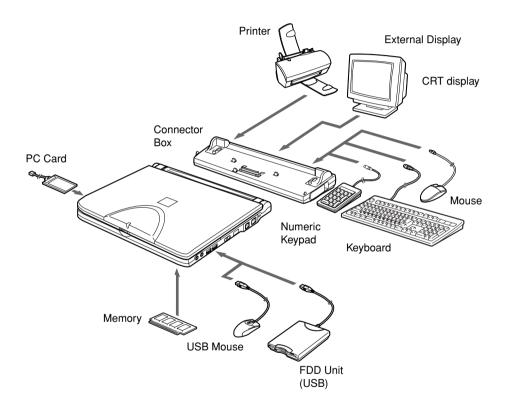
\* If you want to start up your PC from the floppy disk that is set in FDD Unit (USB), it is supported only when doing a recovery using the Recovery CD-ROM Start-up Disk. Note that some models don't support FDD Unit (USB).
