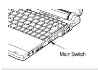
Slide the MAIN switch toward the arrow direction (  $\bigcirc$  side).
