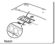
Align the hollow part on the memory and the protrusion of the connector and insert the memory firmly as seen above and turn it down until you can hear snap sound. 6 Attach the RAM Expansion Module Slot Cover.
