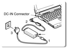
(1)Connect the cord of the AC adapter. (2) Connect the adapter to the DC-IN connector
