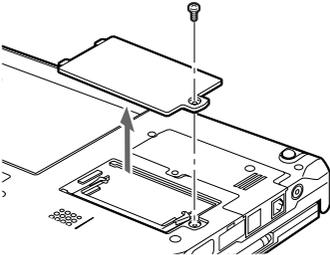
Take out the screws on the bottom of the computer main unit and remove the cover of the expansion RAM module slot.
