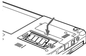
Align the notch of the expansion RAM module with the projection on the connector, insert firmly diagonally from above and push down until the module clicks into place.
