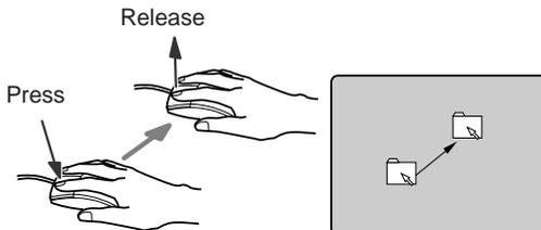
Move the mouse pointer with the mouse left button held down, then release the button at the desired position.
