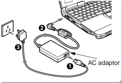
First connect the AC power cord to the AC adaptor (1), next connect the other cord of the AC adaptor to the personal computer's DC-IN connector (2). Lastly, plug the AC power cord into an AC outlet (3).
