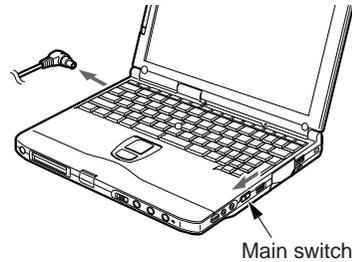
Slide the main switch in the direction of the arrow (to the ○ side).
