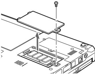
Remove the cover of the expansion RAM module slot on the bottom of the computer main unit.
