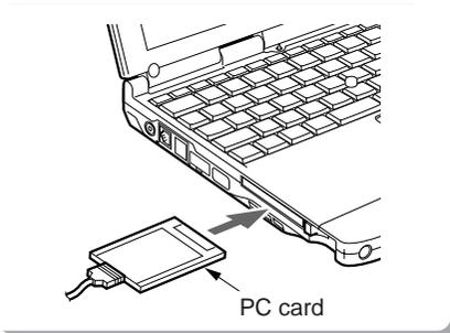
Insert the PC card into the PC card slot with the product name facing upwards.
