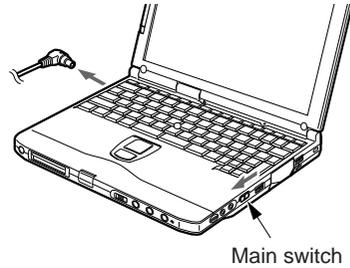
Slide the MAIN switch in the direction of the arrow (toward
