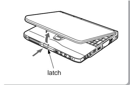
Push the latch to release the lock, then lift the display panel with your hand.
