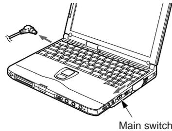
Slide the main switch in the direction of the arrow (to the
