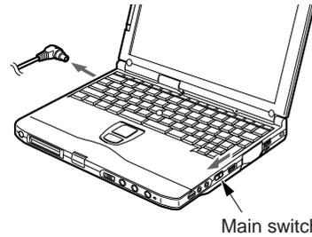
Slide the main switch in the direction of the arrow (to the
