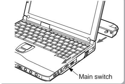
Slide the main switch in the direction shown by the arrow (toward  $\bigcirc$ ) to attach the connector box.
