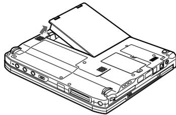
Raise the two latches on the internal battery pack while holding them, and remove the internal battery pack.
