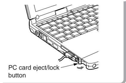
Pull out the PC card eject/lock button completely and then tilt it down to lock the PC card with the fastener.
