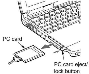
Press the PC card eject/lock button to eject the PC card.
