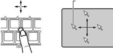
The small arrow (mouse pointer) on the screen moves as you move the stick with a fingertip. Move the stick to and fro, and to the right and left to see how the pointer moves on the screen.
