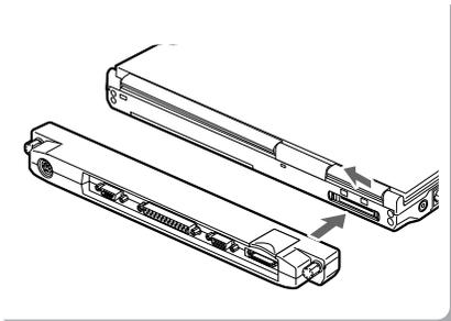
Open the cover of the connector box connector located on the rear side of the personal computer, and tightly connect the connector box to the personal computer by their respective connectors.
