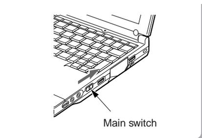
Power is supplied from the AC adaptor or the battery, the power comes on, and the POST starts. Also, the ① etc. on the status indicator L
