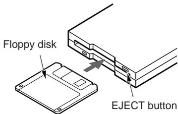
Insert the floppy disk with the label upwards and the shutter side first until the EJECT button springs out.
