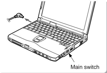
Slide the main switch in the direction of the arrow (O side). Disconnect the AC adaptor.
