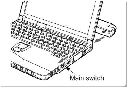
Slide the main switch in the direction of the arrow (○ side).
