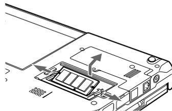
Open the hooks on both sides that retain the expansion RAM module to the left and right, then remove the expansion RAM module from the slot.
