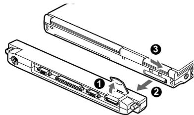
Raise the connector box release lever and detach the connector box. After this, close connector cover.
