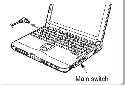
Slide the MAIN switch in the direction of the arrow (toward
