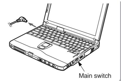
Slide the main switch in the direction of the arrow (I side).
