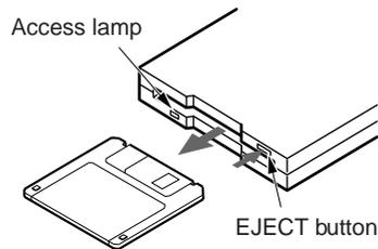
Check that the floppy disk unit's access lamp is out, then press the EJECT button.
