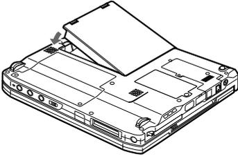
Connect the connector of the new internal battery pack to the connector of your personal computer, and then insert and latch the battery pack.
