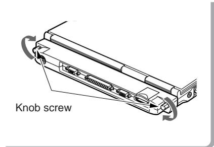
Tighten the right and left knob screws evenly to lock the connector box.
