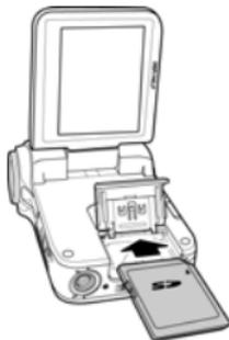
3. Lower and press the SD card slot cover into place.
