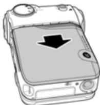
2. Insert the three AAA-type batteries as shown.
