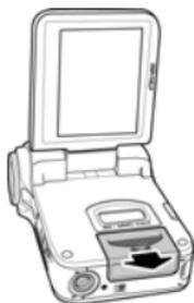
2. Insert an SD card, making sure the contacts are facing downwards.
