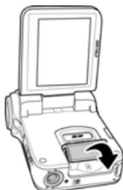
4. Slide the SD card slot cover in to close it.
