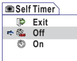
After the self timer is turned on, the camera will have ten seconds delay before taking a picture when the **Record/Shutter** (S) button is pressed. After the shutter fires, the self timer will be automatically disabled.
