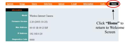
The Information table provides detailed information of the IPCam SECURE300, such as the Model Name, Firmware Version, Mac Address, and IP Address.
