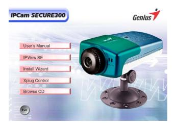
To install the IPView SE application click the "IPView SE" button to activate the installation procedure for the application program.
