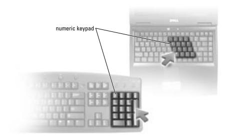
The numeric keypad functions like the numeric keypad on an external keyboard. Each key on the keypad has multiple functions. The keypad numbers and symbols are marked in blue on the right of the keypad keys. To type a number or symbol, hold down <Fn> and press the desired key.
