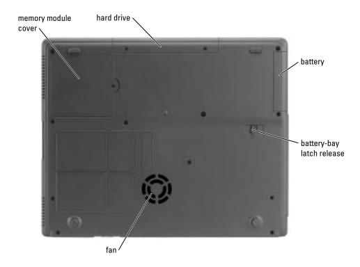
**MEMORY MODULE COVER** — Covers the compartment that contains the memory module(s).
