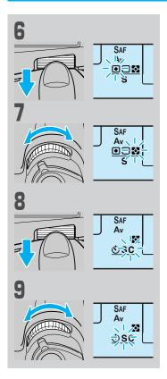
**6** Turn the R dial in the direction of the arrow to display "Metering mode details".
