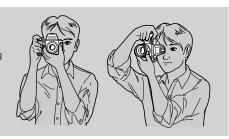
It is important to hold the camera firmly in order to achieve sharp photographs. Unsharp photographs are often due to camera shake caused by the photographer's abrupt motion when taking a picture.
