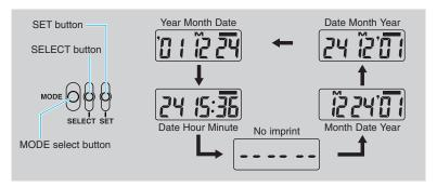
The date and time may be imprinted during photography in cameras fitted with the data back. The separately available Contax Data Back D-11 may be fitted to cameras not supplied with this option.
