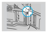
The camera back can be removed and replaced with the separately available D-11 data back (page 96). Remove the camera back by pressing down on the release pin.
