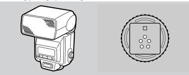
The TLA360 flash has a guide number 36 (ISO 100/35 mm lens angle of view). When used with this camera it offers the six functions described below in addition to regular TTL auto flash photography.
