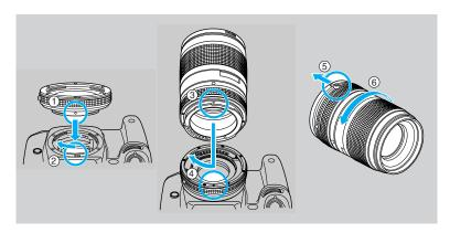
This adapter allows the use of Contax 645 System lenses with the Contax NX. Usable with all NX models.
