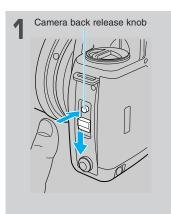
Open the camera back by lifting the camera back release knob while sliding the camera back opening lever downwards.
