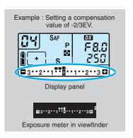
The set compensation appears in the display panel, and the compensation and the "+/-" mark are displayed in the exposure meter in the viewfinder.
