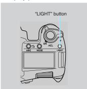
The display panel has an illumination function. Press the "LIGHT" button once to light the display panel, and press it again to extinguish it. The panel is cleared automatically after 16 seconds.
