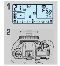
Fit the flash to the camera, select "M" as the exposure mode, and set the shutter speed to a maximum of "X125".
