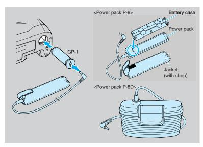
The Power pack P-8 is an external power supply using four 1.5V LR6/AA NiH batteries or four 1.2V LR6/AA Ni-Cd batteries. This pack allows the camera to be used with a remote power supply kept in a warm place. This prevents loss of battery performance due to the influence of cold working conditions.
