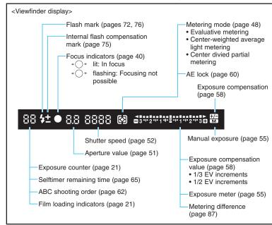
The display in the viewfinder incorporates a variety of information - as well as the focus, aperture, and shutter speed, it also shows the exposure meter and exposure counter.
