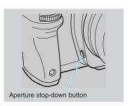
When a lens is focused on the subject, objects within a range in front of, and behind, the subject are also in focus. This range is referred to as the "depth of field". The aperture remains fully open in the viewfinder, however when the aperture stop-down button is pressed the aperture is closed down to the previously set value to allow checking of the depth of field and the fuzziness of the background.
