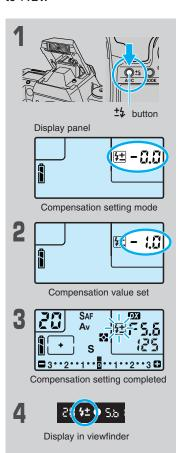
■ Raise the internal flash and press the ½ button to select the light compensation setting mode.
