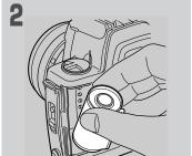
Insert the film at an angle as shown on the diagram.
