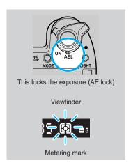
Point the camera so that the center of the viewfinder is on the area for which the exposure is required, turn the main switch "ON" and select "AEL". The exposure is then locked (AE lock).
