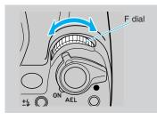
The flash intensity is compensated in conjunction with the camera's F dial exposure compensation with TTL auto flash photography. Use the F dial to adjust flash intensity for maximum effect.
