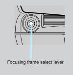
This camera has five focusing frames: the frame at the center of the picture, and four peripheral frames positioned diagonally.
