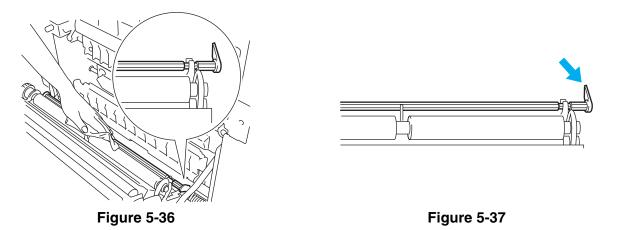
**4** Clean the transfer roller unit and the transfer roller guide with a dry soft cloth to prevent paper jams.
