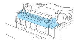
The fusing unit is marked with the caution label. Please do NOT take off or damage the label.
