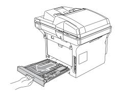
2 Pull the jammed paper out of the machine or the duplex tray.
