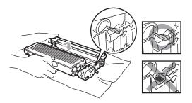
5 Put the drum unit and toner cartridge assembly back in the machine.
