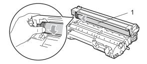
4) When you find the substance on the drum surface that matches the print sample, gently dab the surface of the OPC drum with a cotton swab that is lightly dampened with isopropyl alcohol.
