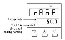
Fig. 2. Ramp Control Screen.
