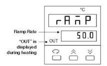
Fig. 2. Ramp Control Screen.
