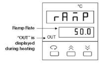
Fig. 2. Ramp Control Screen.
