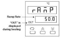
Fig. 2. Ramp Control Screen.
