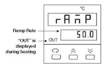
Fig. 2. Ramp Control Screen.
