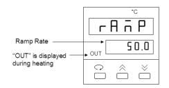
Fig. 2. Ramp Control Screen.
