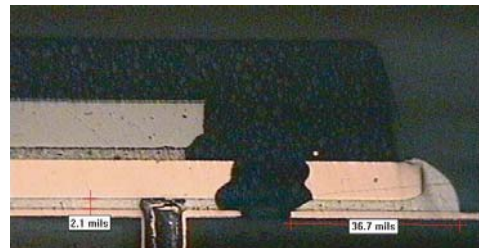
81% paste coverage, encroached via, 2.1 mil standoff
