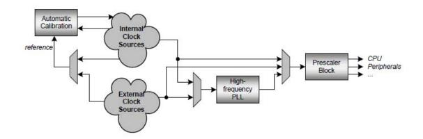
There are five internal clock sources (including the internal PLL), ranging from an ultra low-power (ULP) 32 kHz RC oscillator to a 32 MHz factory-calibrated ring oscillator with auto-calibration features. All sources except the ULP 32 kHz RC oscillator can be used for the main system clock.
