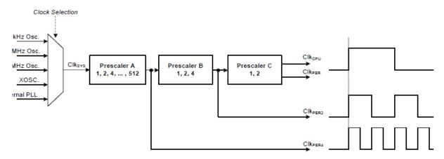
The A, B and C prescalers gives us even more flexibility in the input clock selection. By using any of the available clock sources together with the prescalers, we are able to run the peripherals and CPU at various frequencies just by reconfiguring the A, B and C prescalers.
