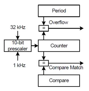
The input clock for the RTC can be the 32 kHz clock directly or a 1 kHz prescaled version of the 32 kHz clock. In addition the RTC has a separate prescaler block in order to choose accuracy over long time-out periods. With a maximum resolution of  $30.5 \ \mu$ s, time-out periods range up to 2000 seconds. With a resolution of 1 second, the maximum time-out period is over 18 hours (65536 seconds).
