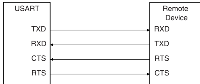
Figure 29-16. Connection with a Remote Device for Hardware Handshaking
