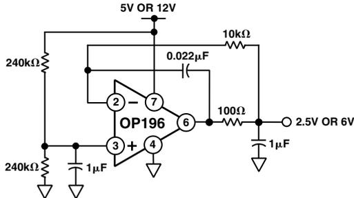
Figure 5. A Micropower False-Ground Generator
