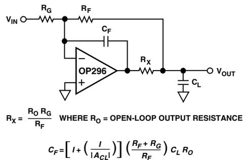
Figure 4. In-the-Loop Compensation Technique for Driving Capacitive Loads
