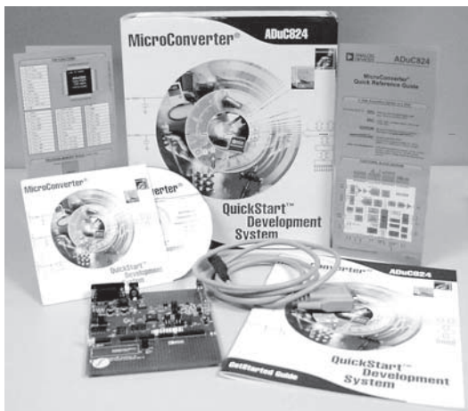
Figure 65. Components of the QuickStar Development System
