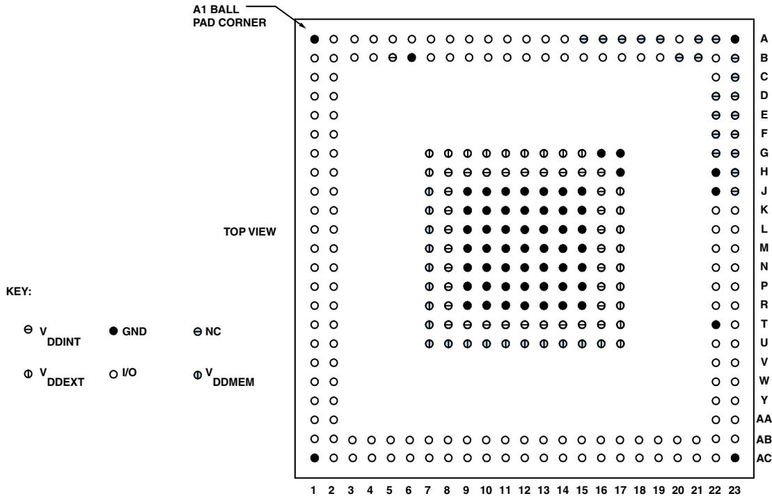
Figure 65. 289-Ball CSP\_BGA Ball Configuration (Top View)
