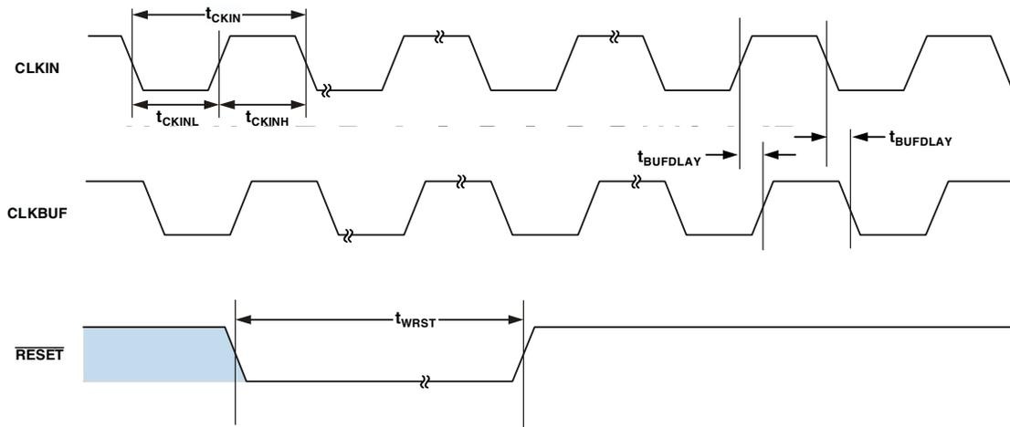
Figure 9. Clock and Reset Timing
