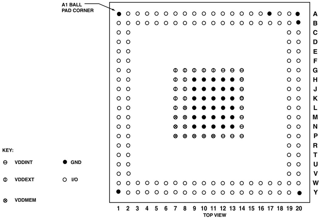
Figure 67. 208-Ball CSP\_BGA Ball Configuration (Top View)
