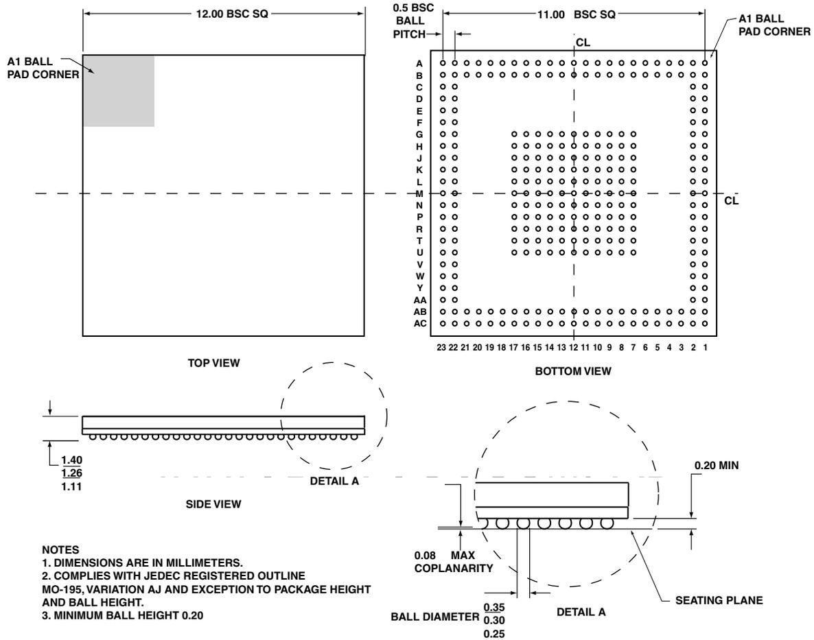
Figure 69. 289-Ball CSP\_BGA (BC-289-2)
