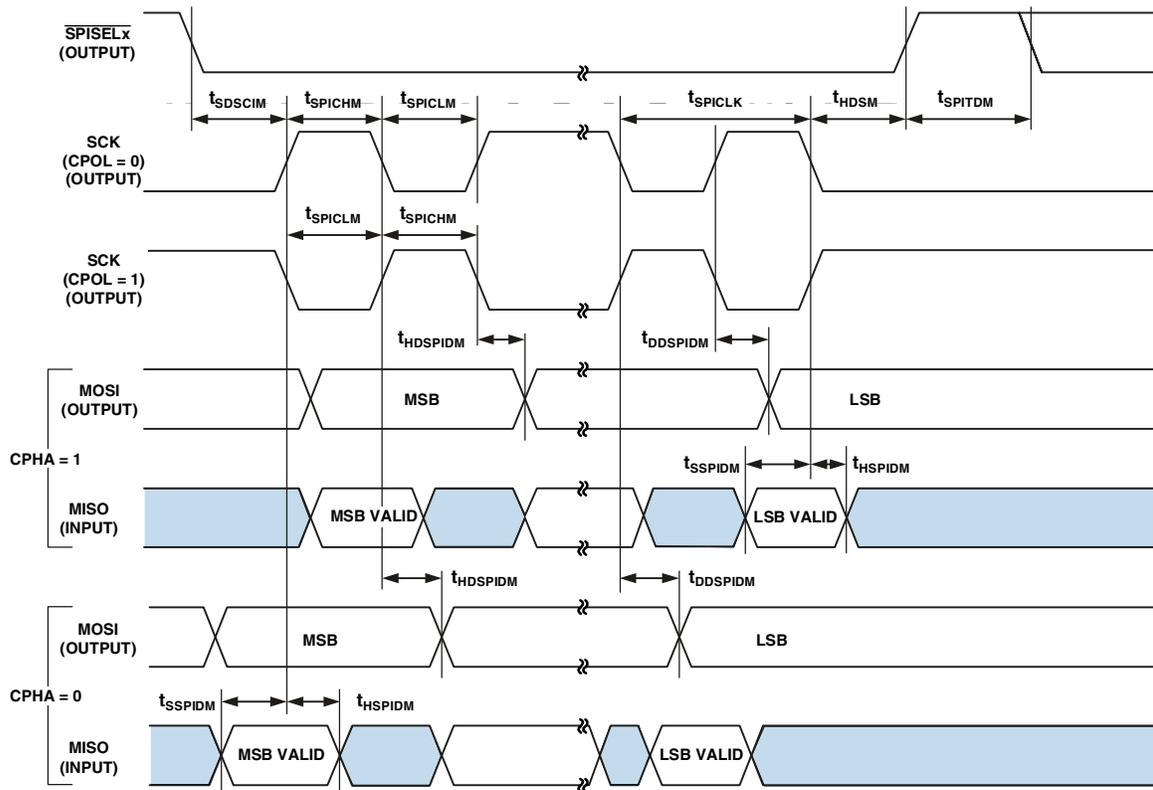
Figure 25. Serial Peripheral Interface (SPI) Port—Master Timing
