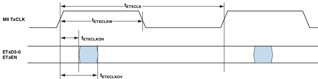
Figure 35. 10/100 Ethernet MAC Controller Timing: MII Transmit Signal
