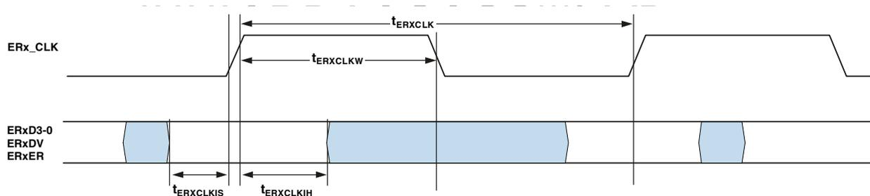
Figure 34. 10/100 Ethernet MAC Controller Timing: MII Receive Signal
