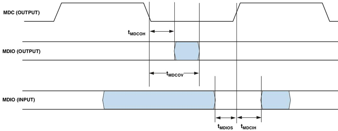
Figure 39. 10/100 Ethernet MAC Controller Timing: MII Station Management
