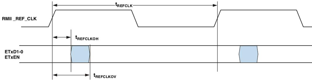
Figure 37. 10/100 Ethernet MAC Controller Timing: RMI Transmit Signal
