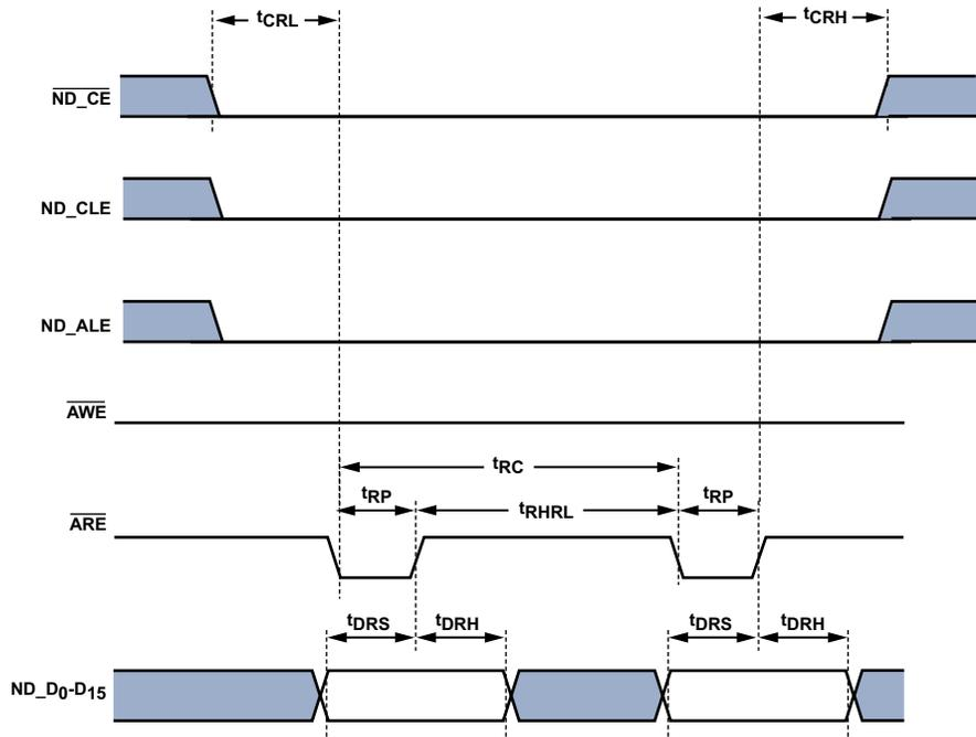
Figure 15. NAND Flash Controller Interface Timing - Data Read Operation
