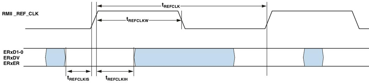
Figure 36. 10/100 Ethernet MAC Controller Timing: RMI Receive Signal
