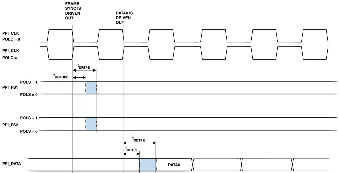
Figure 22. PPI GP Tx Mode with Internal Frame Sync Timing
