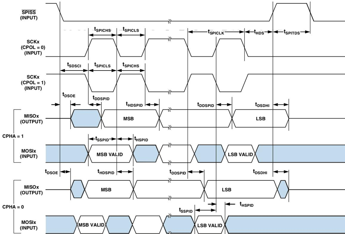
Figure 26. Serial Peripheral Interface (SPI) Port—Slave Timing
