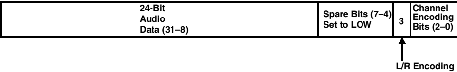
Figure 7-5. FIFO Data Packing for Right-Justified
