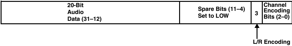
Figure 7-6. FIFO Data Packing for Right-Justified (20-Bit Data)
