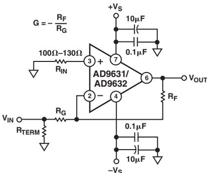
Figure 4. Inverting Operation
