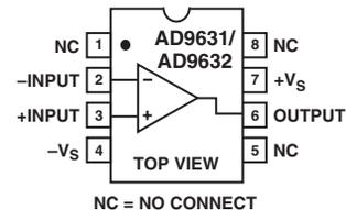
A proprietary design architecture has produced an amplifier that combines many of the best characteristics of both current feedback and voltage feedback amplifiers. The AD9631 and AD9632 exhibit exceptionally fast and accurate pulse response (16 ns to 0.01%) as well as extremely wide small signal and large signal bandwidth and ultralow distortion. The AD9631 achieves -72 dBc at 20 MHz, and 320 MHz small signal and 175 MHz large signal bandwidths.
