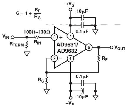
Figure 3. Noninverting Operation
