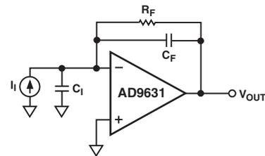
Figure 5. Transimpedance Configuration
