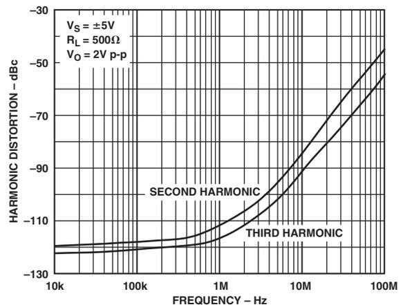
Figure 1. AD9631 Harmonic Distortion vs. Frequency,  $G = +1$
