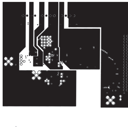
Figure 16. PCB Power Layers—Layers 3 and 4
