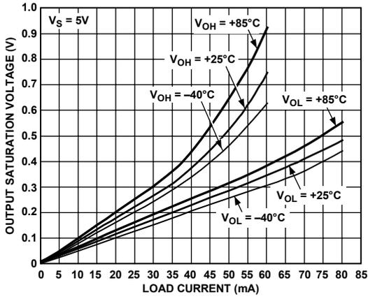
Figure 31. AD8051/AD8052 Output Saturation Voltage vs. Load Current
