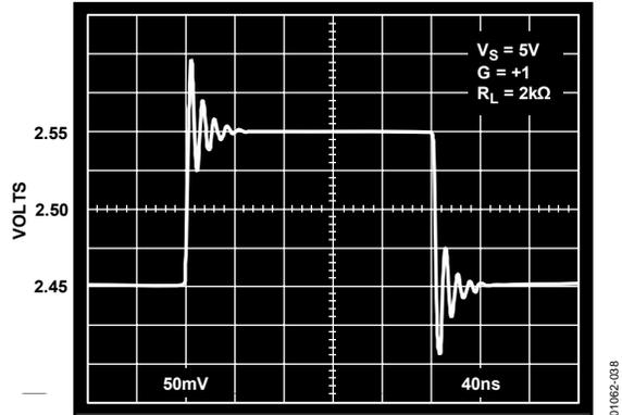
Figure 38. AD8054 100 mV Step Response;  $V_S = 5V$ ,  $G = +1$
