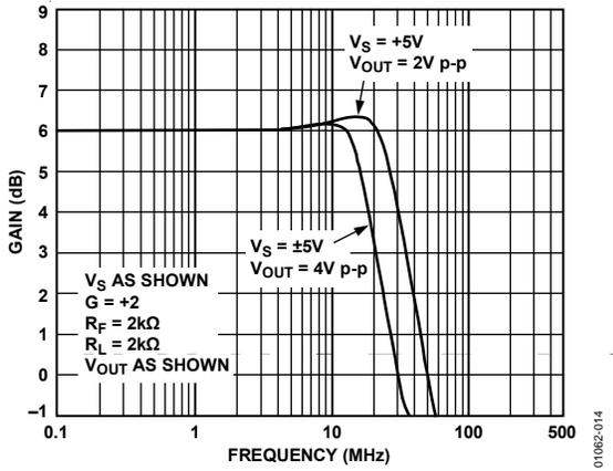
Figure 14. AD8051/AD8052 Large Signal Frequency Response;  $G = +2$
