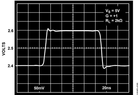
Figure 35. AD8051/AD8052 200 mV Step Response;  $V_S = 5V$ ,  $G = +1$
