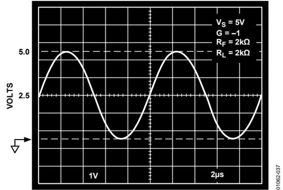
Figure 37. Output Swing;  $G = -1$ ,  $R_L = 2k\Omega$
