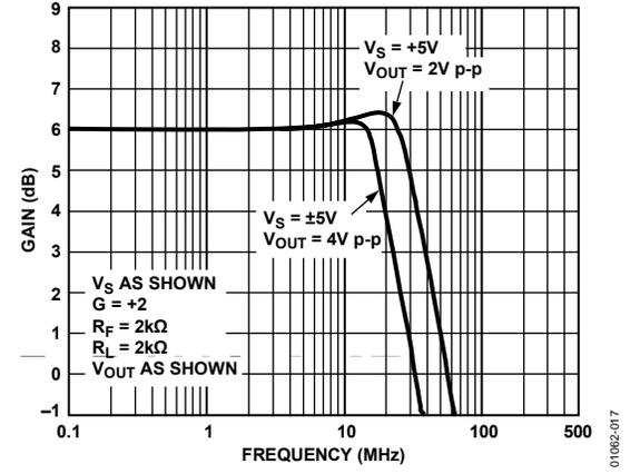
Figure 17. AD8054 Large Signal Frequency Response;  $G = +2$
