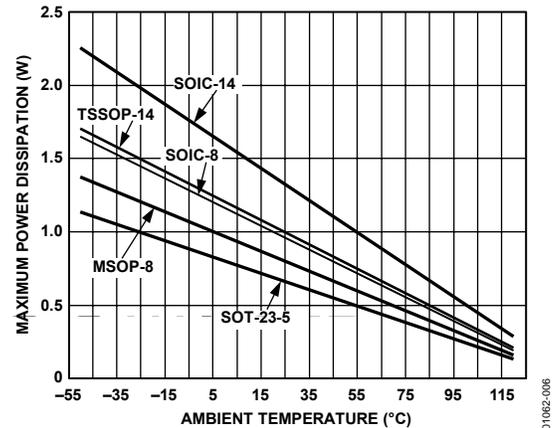
Figure 6. Maximum Power Dissipation vs. Temperature for AD8051/AD8052/AD8054
