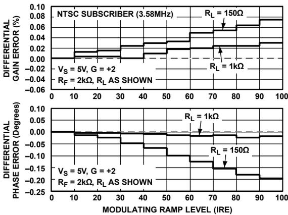
Figure 21. AD8051/AD8052 Differential Gain and Phase Errors
