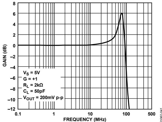
Figure 42. AD8051/AD8052 Closed-Loop Frequency Response;  $C_L = 50\text{ pF}$
