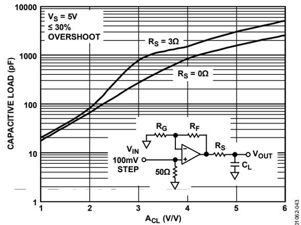
Figure 44. AD8051/AD8052 Capacitive Load Drive vs. Closed-Loop Gain
