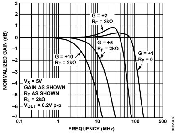
Figure 7. AD8051/AD8052 Normalized Gain vs. Frequency;  $V_S = 5V$
