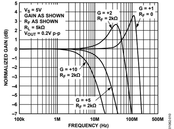
Figure 10. AD8054 Normalized Gain vs. Frequency;  $V_S = 5V$
