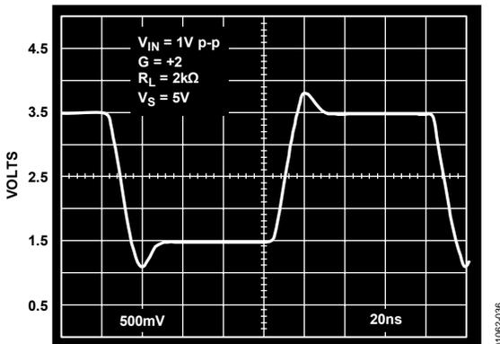
Figure 36. Large Signal Step Response;  $V_S = 5V$ ,  $G = +2$
