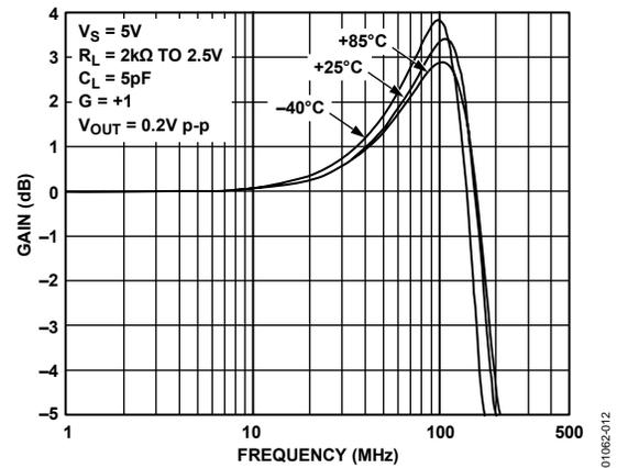
Figure 12. AD8054 Gain vs. Frequency vs. Temperature
