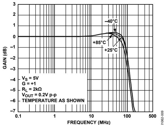
Figure 9. AD8051/AD8052 Gain vs. Frequency vs. Temperature
