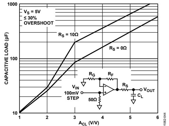
Figure 45. AD8054 Capacitive Load Drive vs. Closed-Loop Gain
