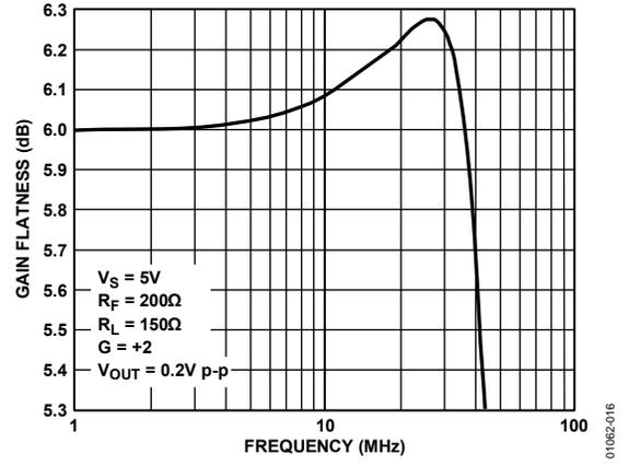
Figure 16. AD8054 0.1 dB Gain Flatness vs. Frequency;  $G = +2$
