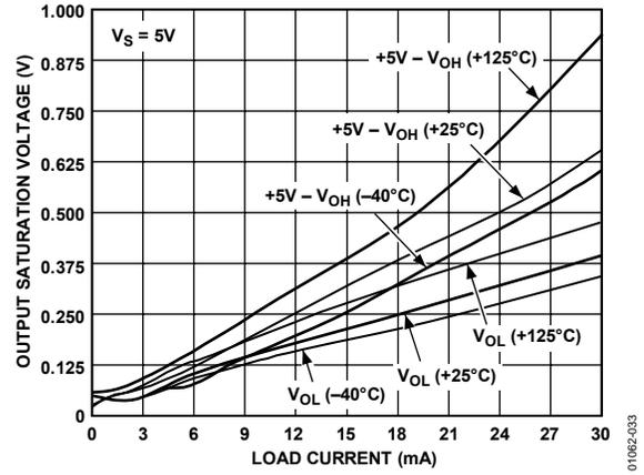
Figure 33. AD8054 Output Saturation Voltage vs. Load Current
