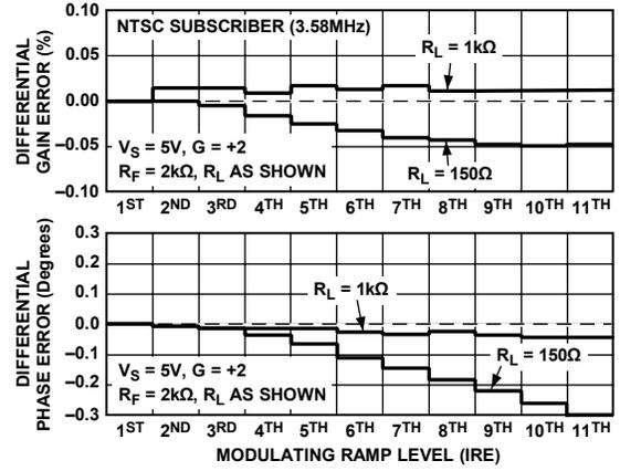
Figure 24. AD8054 Differential Gain and Phase Errors
