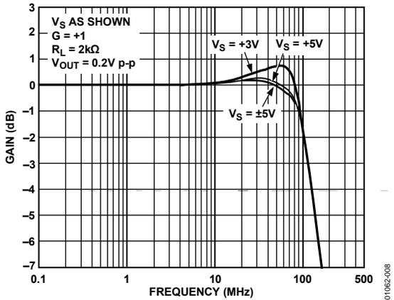
Figure 8. AD8051/AD8052 Gain vs. Frequency vs. Supply
