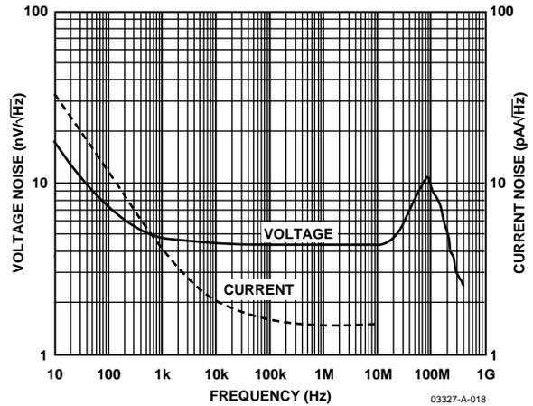
Figure 19. Voltage and Current Noise vs. Frequency
