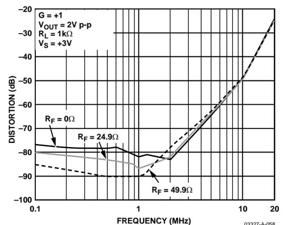
Figure 59. SFDR vs. Frequency and Various  $R_F$
