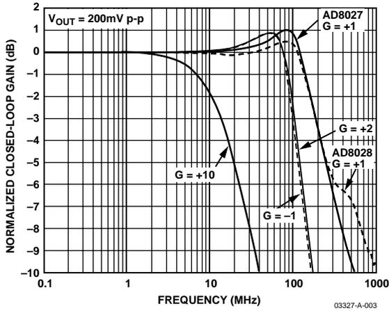
Figure 4. Small Signal Frequency Response for Various Gains
