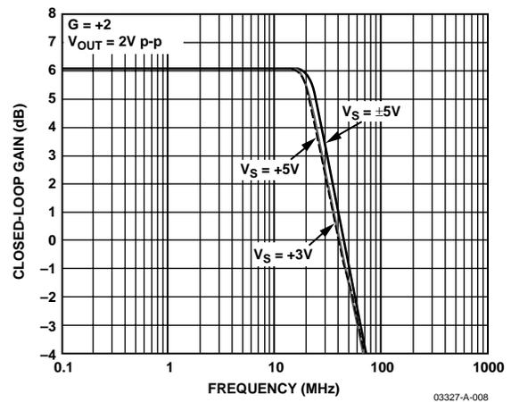
Figure 9. Large Signal Frequency Response for Various Supplies
