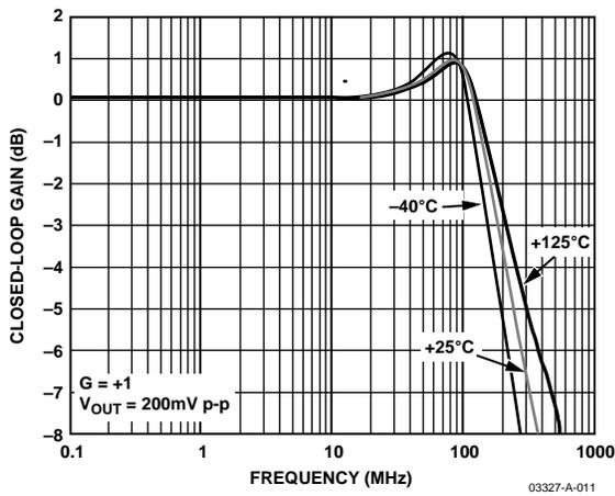
Figure 12. AD8027 Small Signal Frequency Response vs. Temperature
