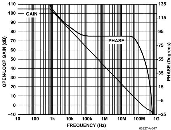
Figure 18. Open-Loop Gain and Phase vs. Frequency
