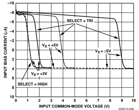
Figure 37. Input Bias Current vs. Input Common-Mode Voltage
