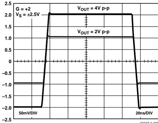
Figure 30. Large Signal Transient Response,  $G = +2$
