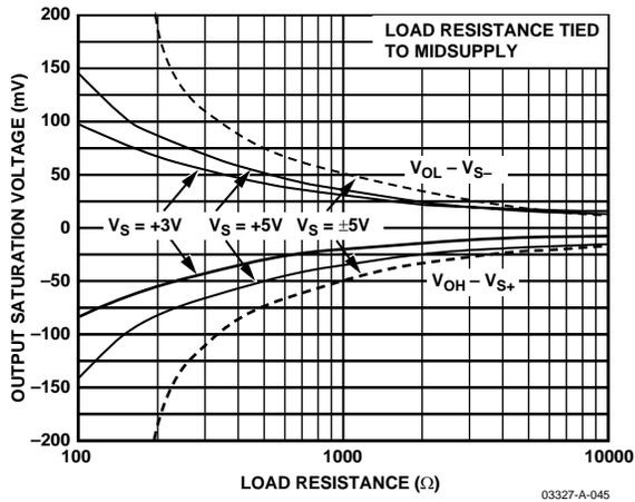
Figure 46. Output Saturation Voltage vs. Output Load
