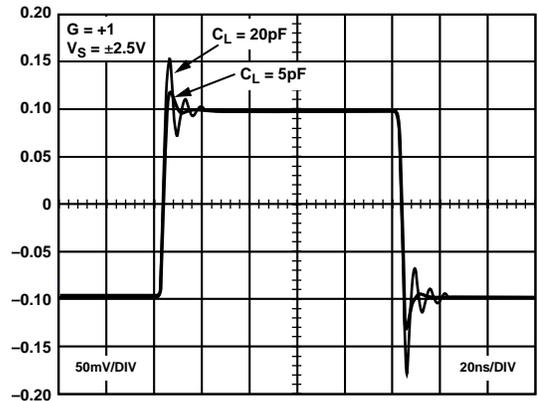
Figure 31. Small Signal Transient Response with Capacitive Load
