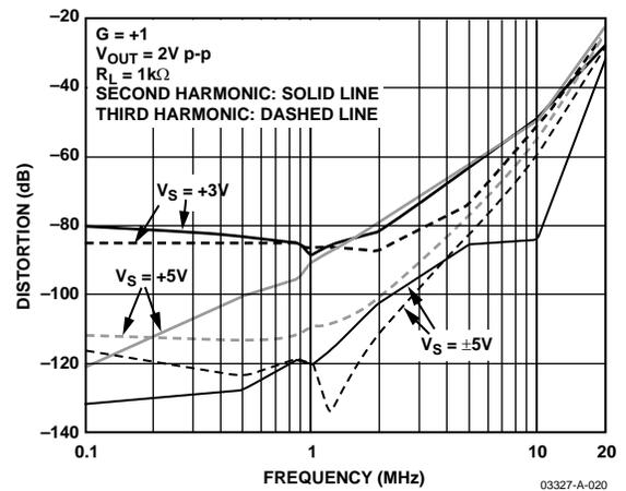
Figure 21. Harmonic Distortion vs. Frequency and Supply Voltage
