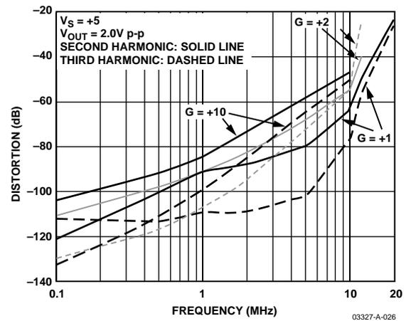
Figure 27. Harmonic Distortion vs. Frequency and Gain
