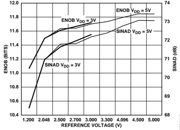
Figure 17. SINAD/ENOB vs. Reference Voltage, Mode 1, 121 kSPS
