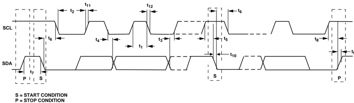
Figure 2. Timing Diagram for 2-Wire Serial Interface
