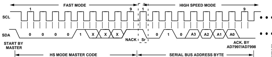
Figure 31. Placing the Part into High Speed Mode
