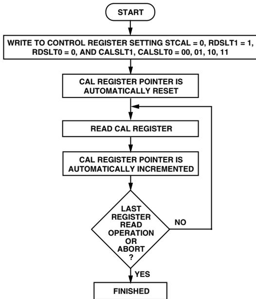
Figure 7. Flowchart for Reading from the Calibration Registers
