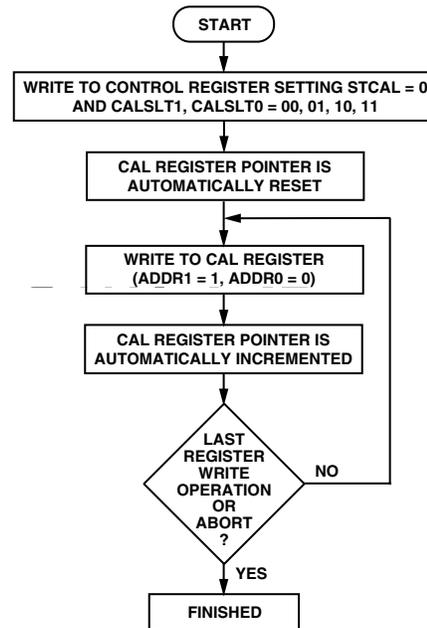
Figure 6. Flowchart for Writing to the Calibration Registers
