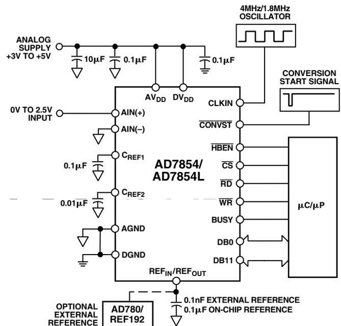
Figure 8. Typical Circuit
