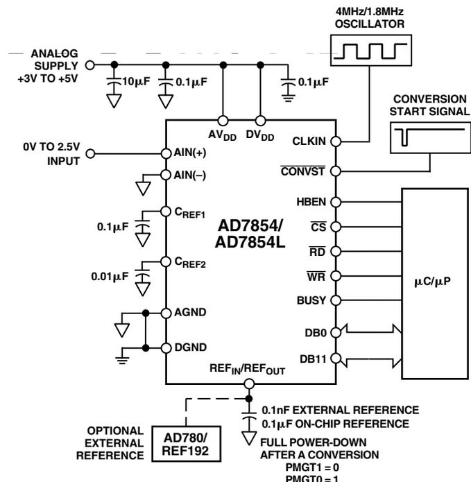
Figure 23. Typical Low Power Circuit
