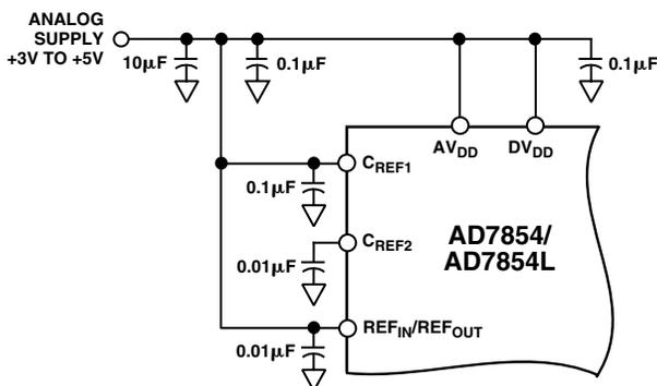
Figure 17. Relevant Connections,  $AV_{DD}$  as the Reference
