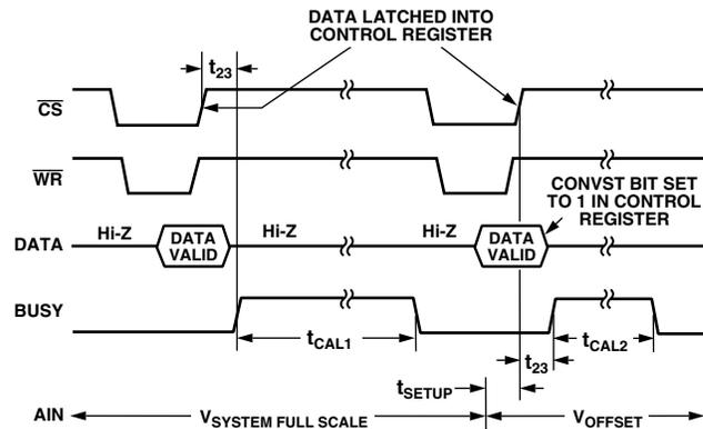
Figure 33. Timing Diagram for Full System Calibration
