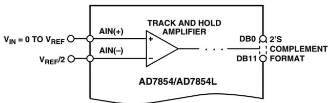
Figure 13.  $\pm V_{REF}/2$  about  $V_{REF}/2$  Bipolar Input Configuration
