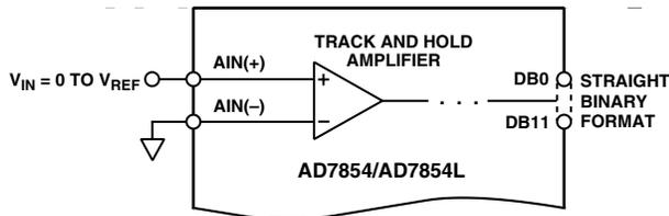
Figure 12. 0 to  $V_{REF}$  Unipolar Input Configuration
