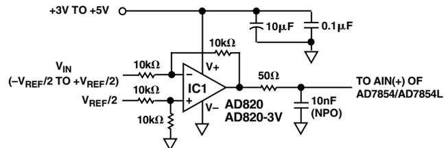
Figure 11. Analog Input Buffering
