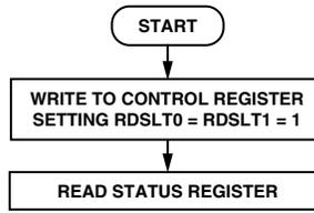
Figure 4. Flowchart for Reading the Status Register
