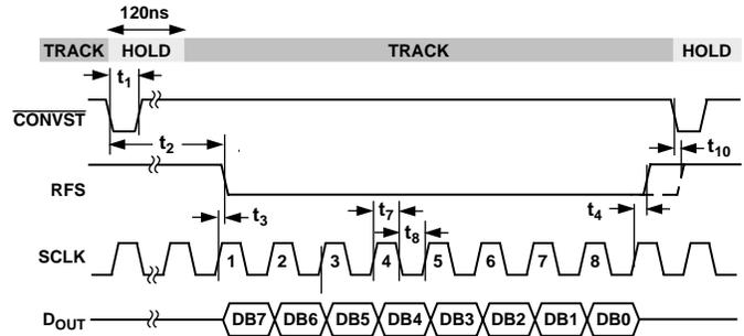
Figure 4. Track-and-Hold Timing
