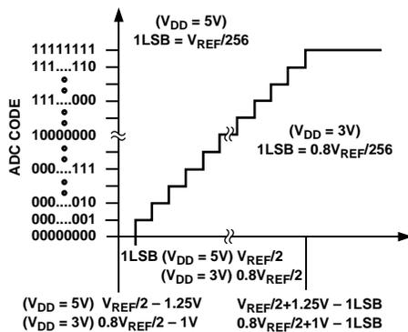
Figure 6. Transfer Characteristic
