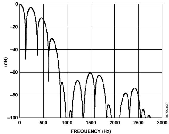
Figure 15. Filter Profile with Update Rate = 242 Hz
