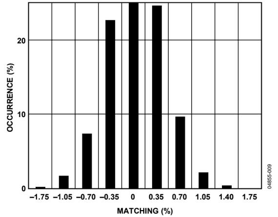
Figure 9. Excitation Current Matching (1 mA) at Ambient Temperature
