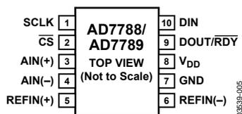
Figure 5. Pin Configuration
