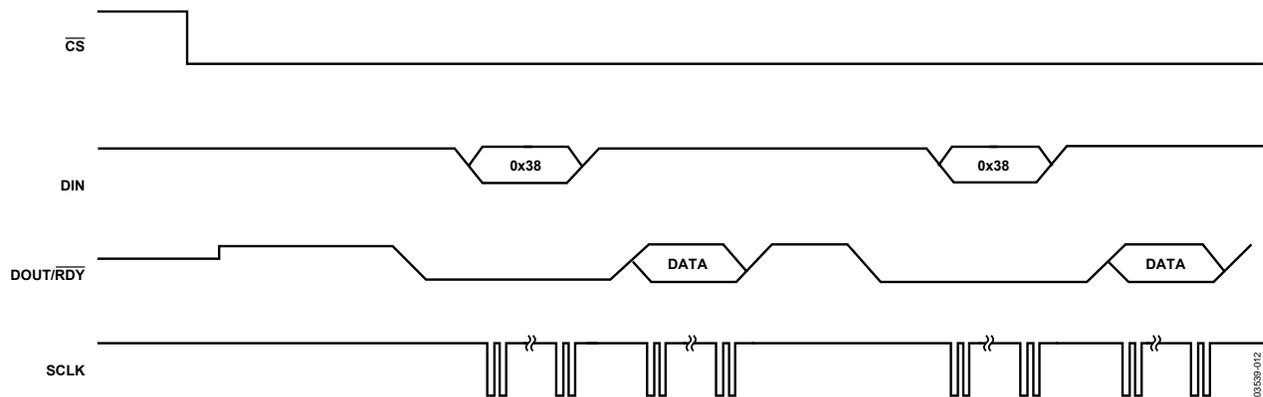
Figure 12. Continuous-Conversion Mode
