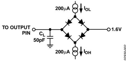
Figure 2. Load Circuit for Digital Output Timing Specifications
