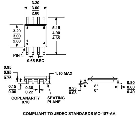
Figure 34. 8-Lead Mini Small Outline Package [MSOP] (RM-8)
