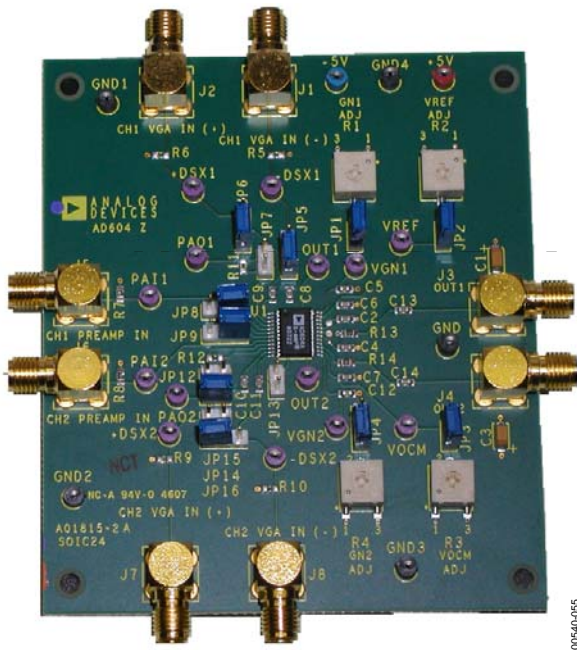
Figure 55. AD604 Evaluation Board Assembly
