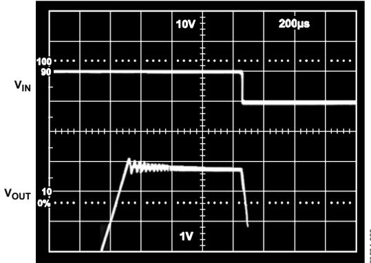
Figure 29. Output Amplifier Step Response,  $C_L = 1 \mu F$
