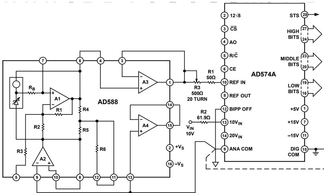
Figure 35. AD588/AD574A Connections
