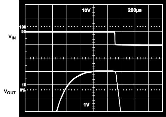
Figure 31. Output Amplifier Step Response Using Figure 30 Compensation
