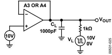
Figure 25. Capacitive Load Transient Response Test Circuit
