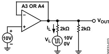
Figure 23. Transient and Constant Load Test Circuit
