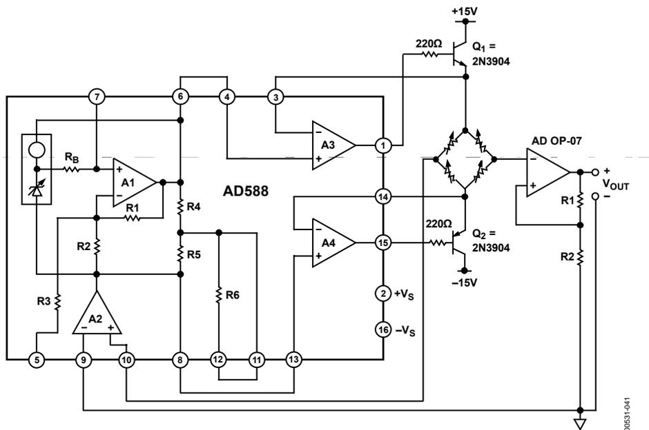
Figure 41. Floating Bipolar Bridge Drive with Minimum CMV
