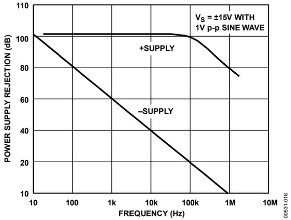
Figure 16. Power Supply Rejection vs. Frequency (A3, A4)
