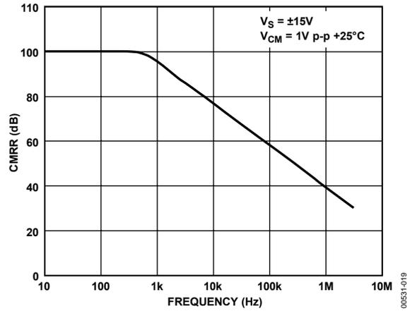
Figure 19. Common-Mode Rejection vs. Frequency (A3, A4)
