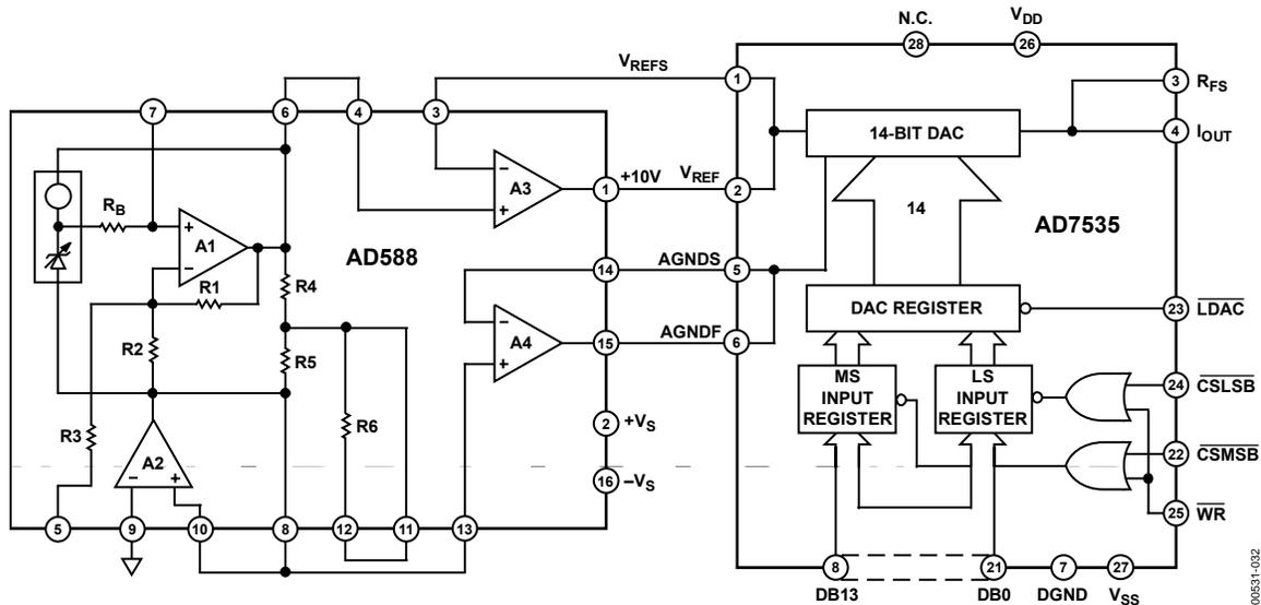
Figure 32. AD588/AD7535 Connections
