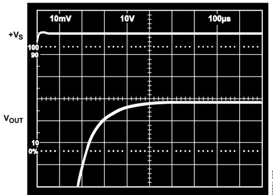
Figure 9. Electrical Turn-On
