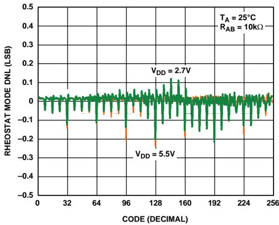
Figure 6. R-DNL vs. Code vs. Supply Voltages
