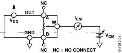
Figure 35. Test Circuit for Common-Mode Leakage Current
