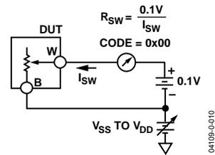
Figure 34. Test Circuit for Incremental On Resistance
