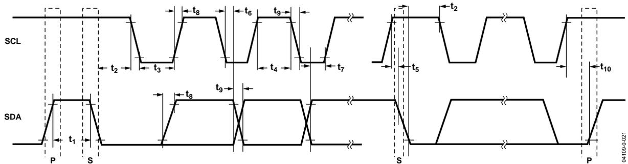
Figure 45. I<sup>2</sup>C Interface Detailed Timing Diagram
