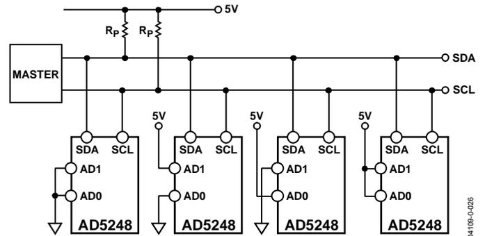
Figure 50. Multiple AD5248 Devices on One I<sup>2</sup>C Bus
