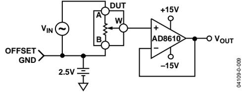
Figure 33. Test Circuit for Gain vs. Frequency
