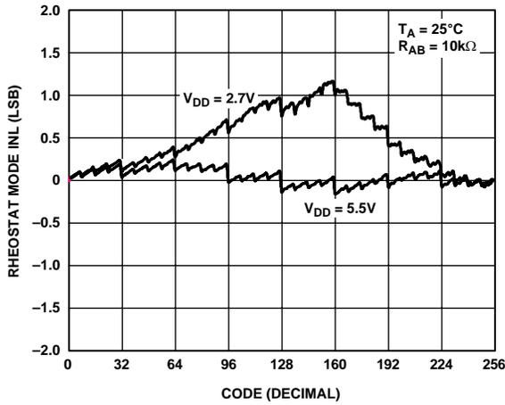
Figure 5. R-INL vs. Code vs. Supply Voltages
