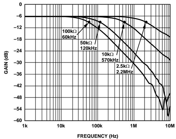
Figure 22. -3 dB Bandwidth @ Code = 0x80
