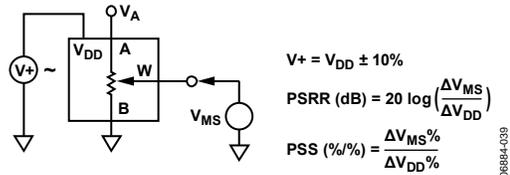
Figure 30. Power Supply Sensitivity Test Circuit (PSS, PSRR)
