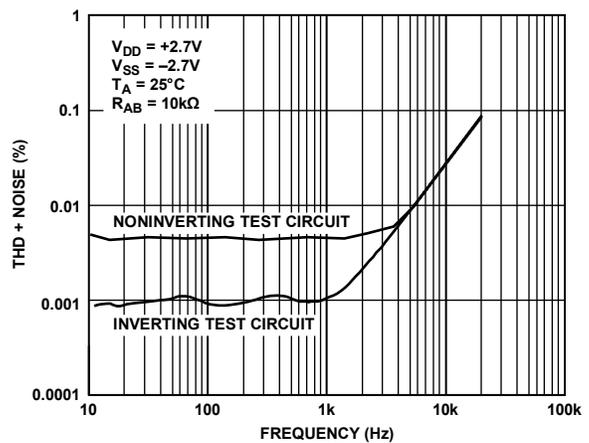
Figure 20. Total Harmonic Distortion Plus Noise vs. Frequency
