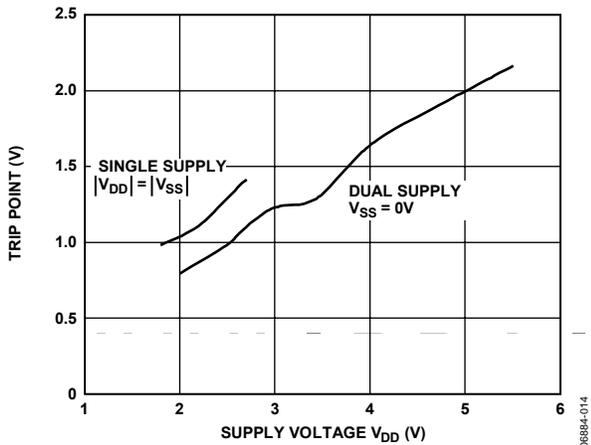
Figure 16. Digital Input Trip Point vs. Supply Voltage
