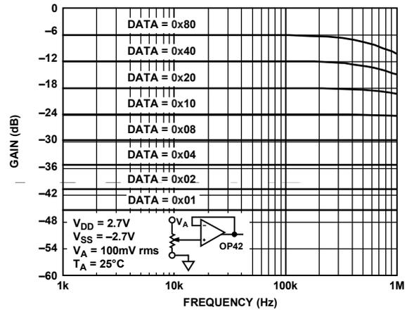
Figure 13. Bandwidth vs. Code, 10 kΩ Version
