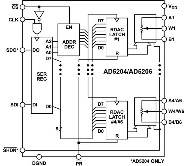
Figure 22. Block Diagram
