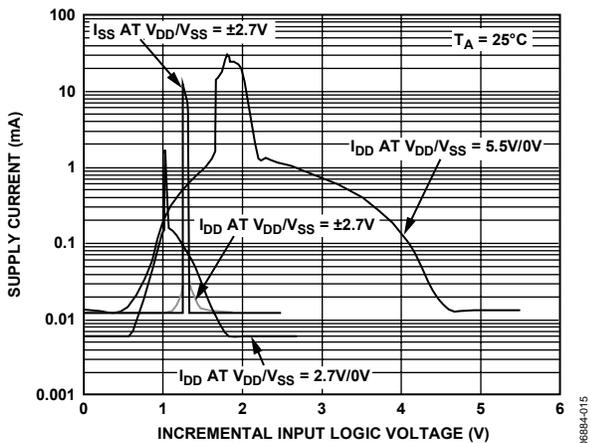
Figure 17. Supply Current vs. Input Logic Voltage
