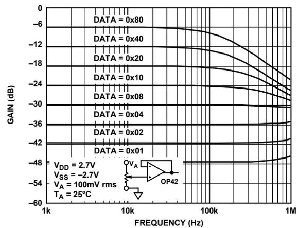
Figure 14. Bandwidth vs. Code, 50 kΩ Version
