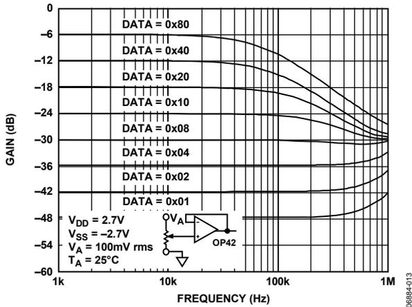
Figure 15. Bandwidth vs. Code, 100 kΩ Version
