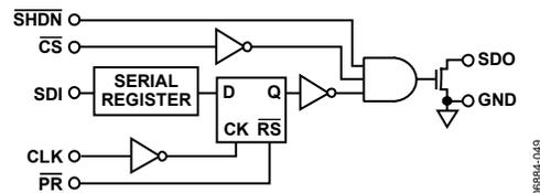
Figure 24. Detail SDO Output Schematic of the AD5204
