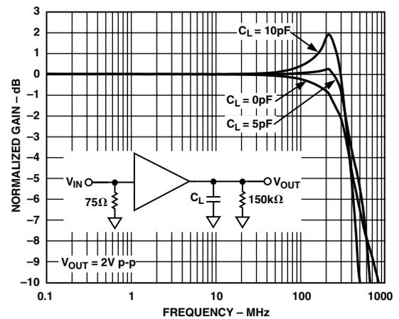
TPC 6. AD8075 Frequency Response vs. Capacitive Load
