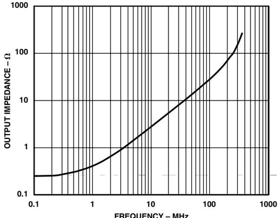
TPC 18. AD8074 Output Impedance vs. Frequency; Enabled
