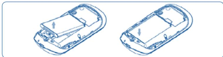
Insert and click the battery into place, make sure battery connecting with battery connector, then close the telephone cover. Unclip the cover, then remove the battery.
