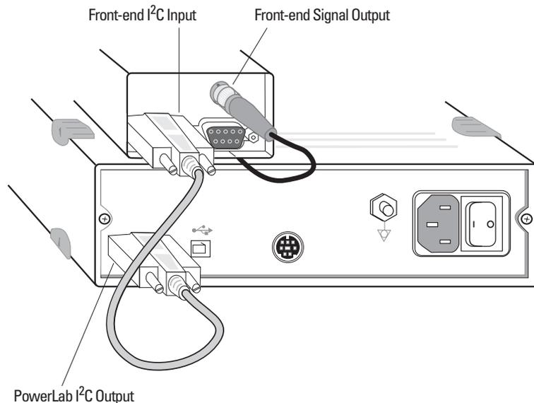
Check that the plugs for the I<sup>2</sup>C bus are screwed in firmly. Check the BNC cable for firm connections as well. Loose connectors can cause erratic front-end behavior, or may cause the front-end to fail to work at all. The BNC cable can be tucked under the front-end to keep it out of the way if desired.
