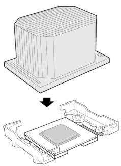
7 Place the heat sink clip (1) so the tab on the clip engages the slot on the heat sink (A).
