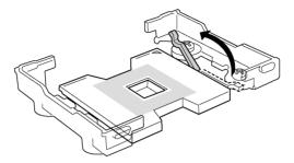
2 Aligning the pins of the processor with the socket, insert the processor into the socket.
