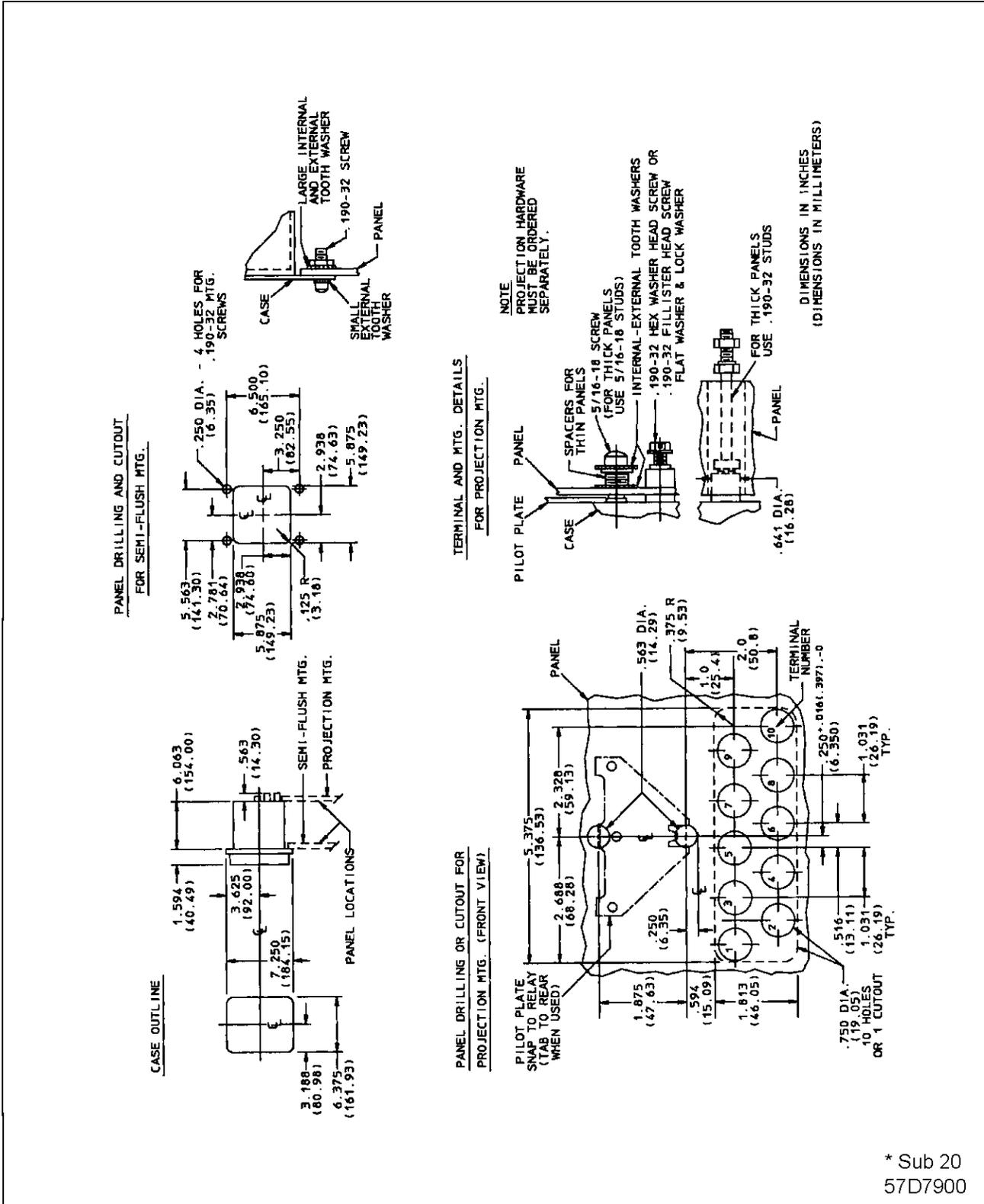
Figure 22: Outline and Drilling Plan for the Type CO Relay
