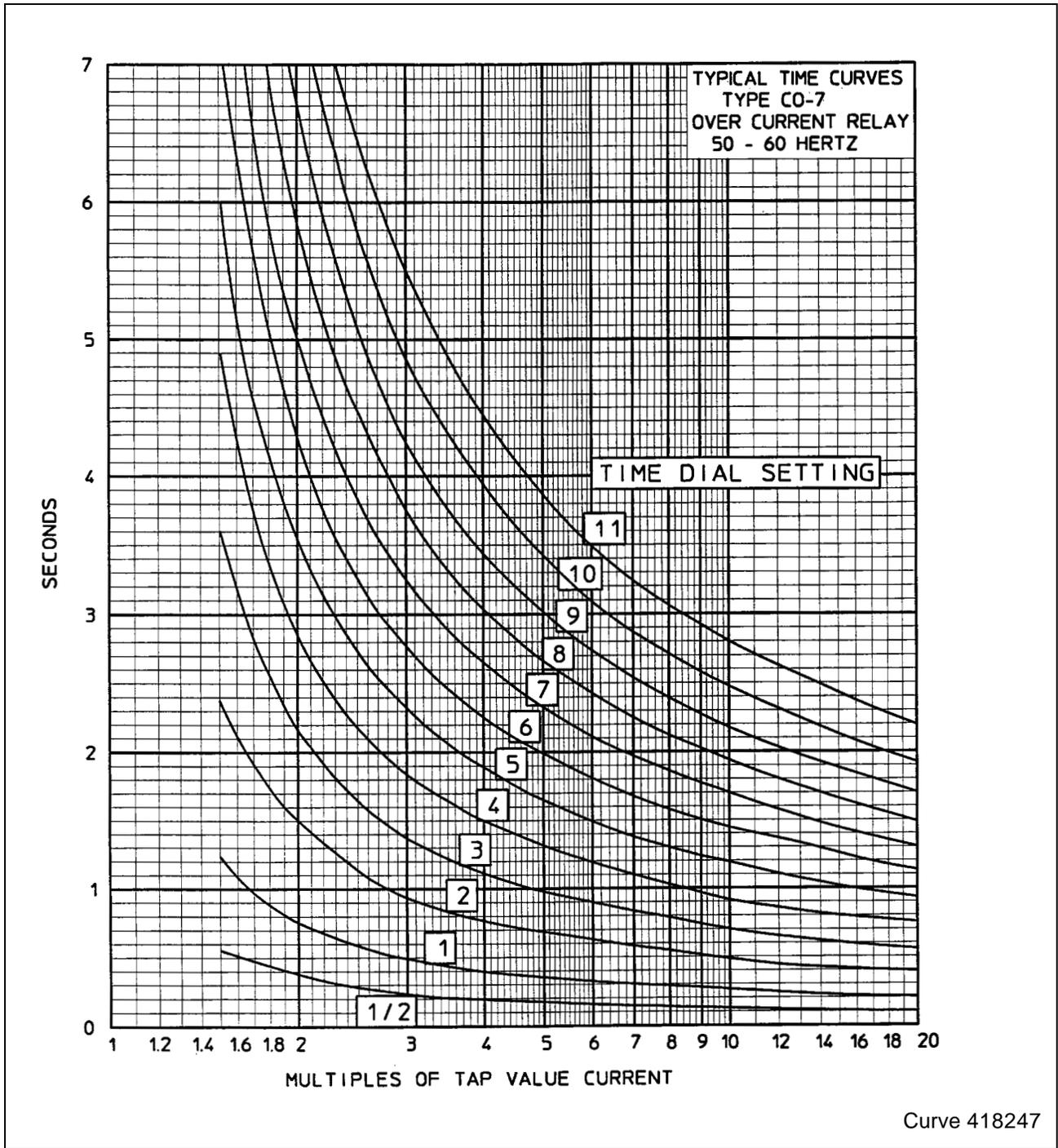
Figure 16: Typical Time Curve of the Type CO-7 Relay
