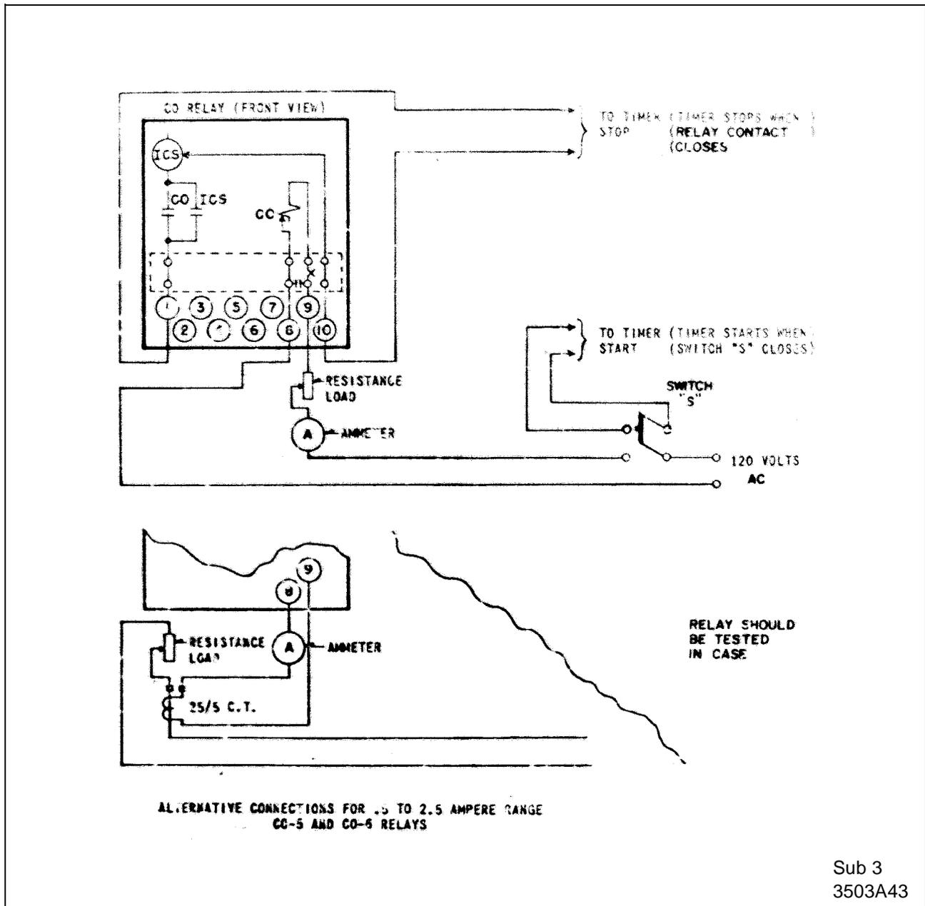
Figure 3: Diagram of Test Connections for Circuit Closing Type CO Relay
