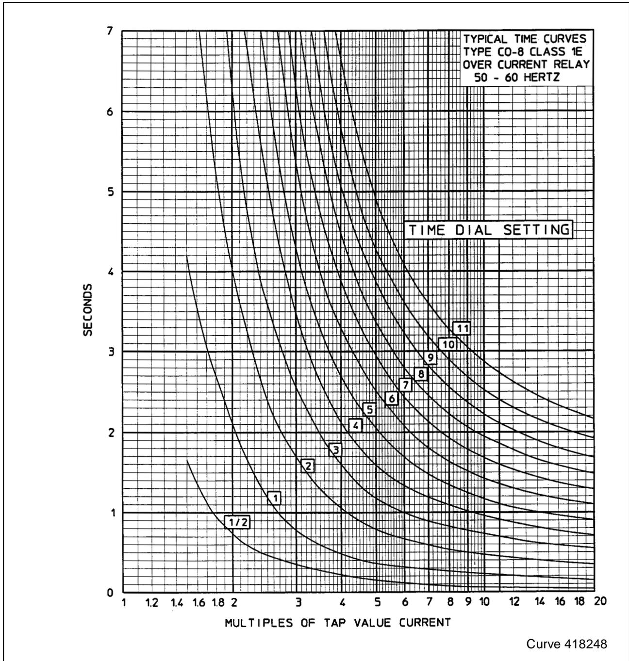
Figure 17: Typical Time Curve of the Type CO-8 Relay
